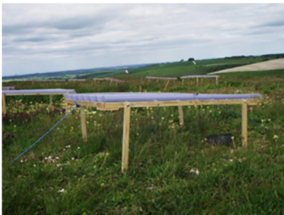
The experimental design using shelters that simulate drought.
